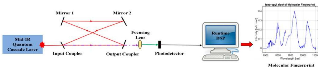
**Figure 1.** Optical diagram for runtime cavity ringdown spectroscopy (rtCRDS) and molecular fingerprinting process.
