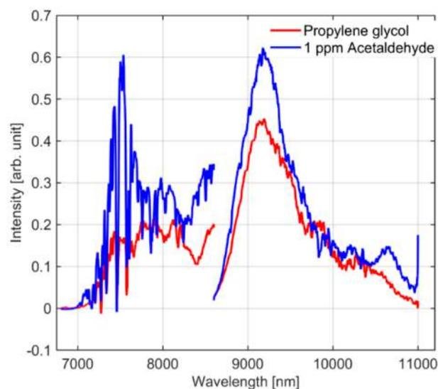
**Figure 3.** An example of the molecular fingerprint of PG aerosol (single puff) vaped by a Juul device and the molecular fingerprint for a 1 ppm acetaldehyde solution.
