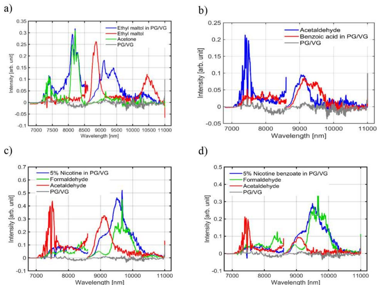
**Figure 5.** Molecular fingerprint of aerosols of additive spikes into 30:70 PG/VG matched with pure chemicals in database: (a) ethyl maltol in PG/VG, pure ethyl maltol, acetone, and PG/VG; (b) benzoic acid in PG/VG, acetaldehyde, and PG/VG; (c) 5% nicotine in PG/VG, acetaldehyde, formaldehyde, and PG/VG; (d) 5% nicotine benzoate in PG/VG, formaldehyde, acetaldehyde, and PG/VG.
