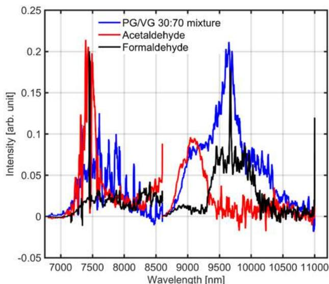
**Figure 4.** Molecular fingerprint spectrum of aerosols collected from three puffs of propylene glycol and vegetable glycerin 30:70 mixture and molecular fingerprint spectra of acetaldehyde and formaldehyde.
