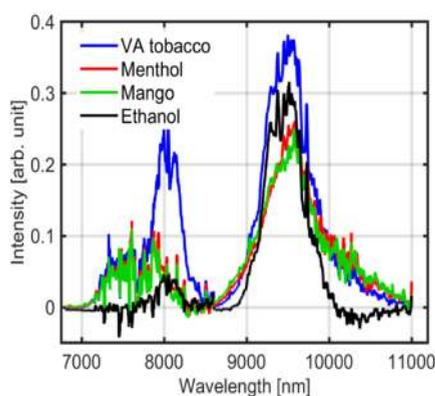
**Figure 7.** Molecular fingerprint spectra of aerosols collected from single puffs of Juul Virginia Tobacco, Menthol, and Mango flavors, superimposed with the molecular fingerprint for ethanol.
