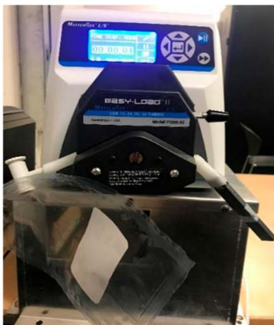
**Figure 2.** Setup for aerosol generation from a Juul device and collection into a 1L Tedlar gas bag using a peristaltic pump.
