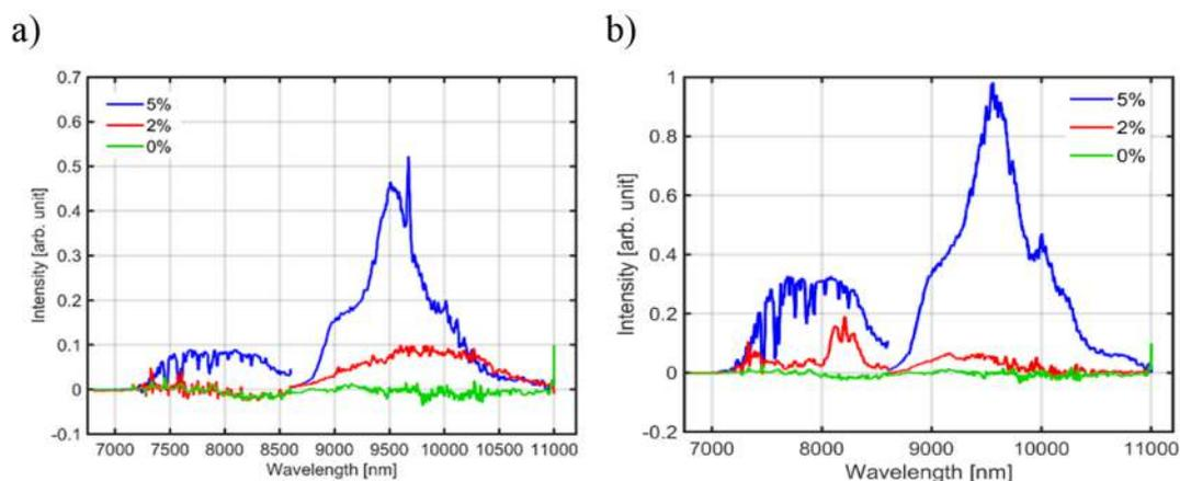
**Figure 6.** Molecular fingerprint spectra of aerosols collected from single puffs of 0, 2, and 5% (a) nicotine and (b) nicotine benzoate salt dissolved in a 30:70 PG/VG mixture.
